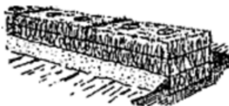
Figure 3: Constructing a straw bale barrier to slow runoff and prevent erosion
